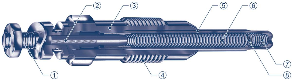
1. **Terminal.** It is a connector with the electric supply. Terminals are predominantly nickel threaded or pin junction.
